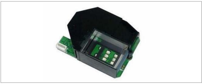
Special electronic circuit is built into FS-88 to do Live Finger Detection (LFD). With appropriate software in PC, user can select this LFD feature so that only live finger's fingerprint will be scanned into PC. Fake fingers made from silicone rubber, play-doh, etc, will be rejected.
